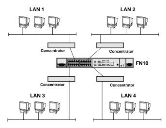
Figure 5-4 Using Firewall Filters to Reduce Multicasts
